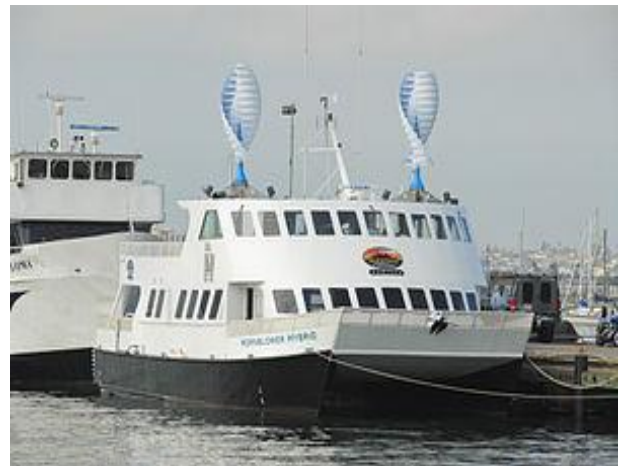
Figure 6.2: Hornblower Hybrid wind, solar and diesel ferry
