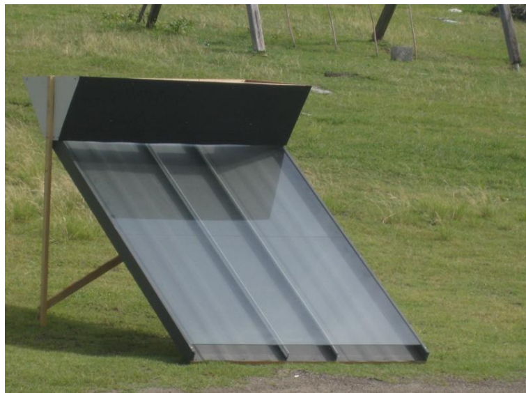
Figure 2.3: Solar drier for fish and fruits (locally constructed)
